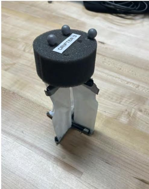
Fig. 11. Passive Drifter
