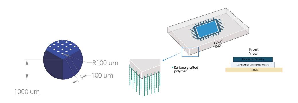
An anisotropic conductive and chronically stable adhesive interface for bioelectronics
