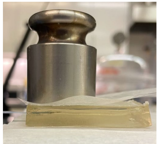
Fig 3. Muscle phantom with inserted microsensor and 200g weight applied on top.
