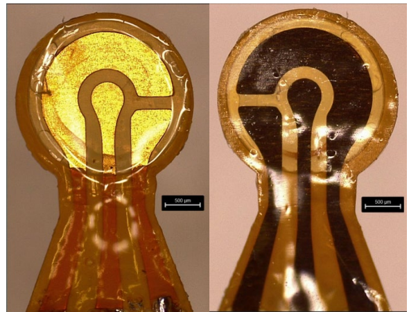
Fig 1. Electrochemical microsensor with SU-8 spacer on the front (left) and PDMS backing on the back (right).
