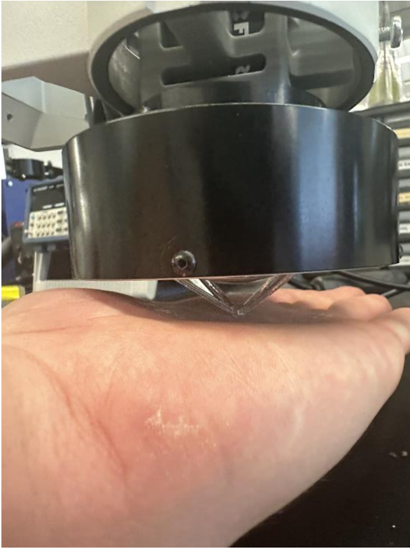
Fig. 4 iPPG Experimental Setup to Capture Force Induced Changes in Cutaneous Blood Volume
