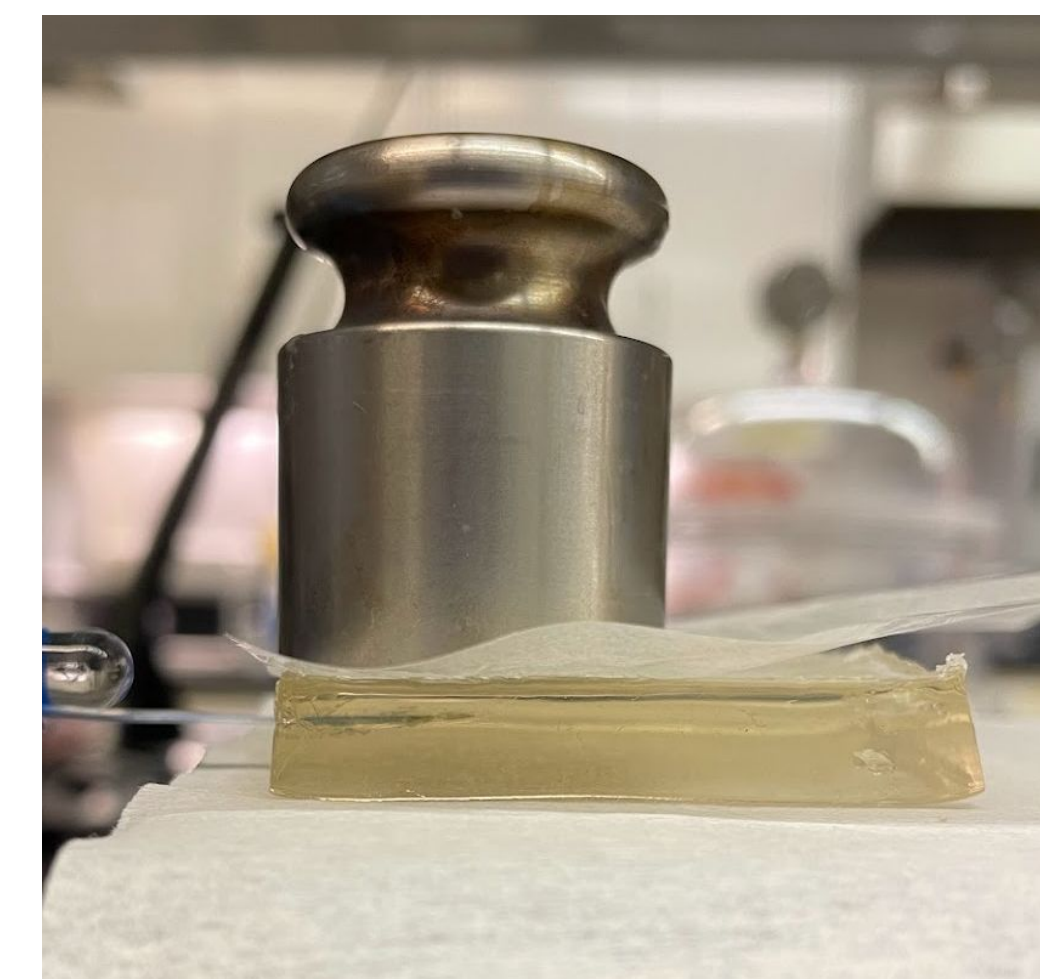
Fig 4. Muscle phantom with inserted sensor undergoing applied external load
