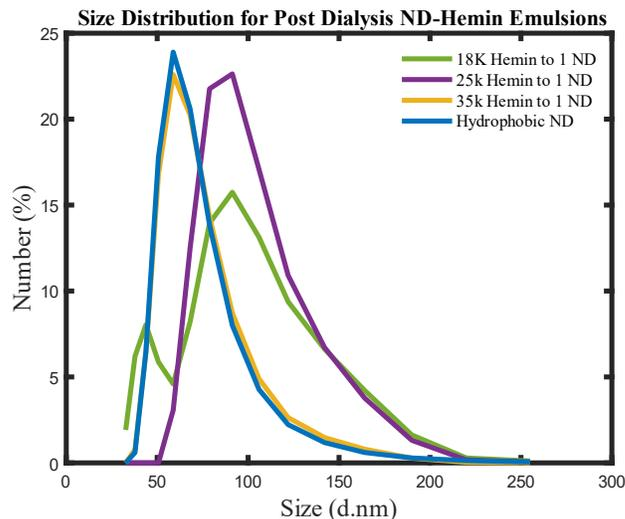
Figure 6. Size distribution for post-dialysis nanodiamond-hemin emulsions measured via dynamic light scattering.
