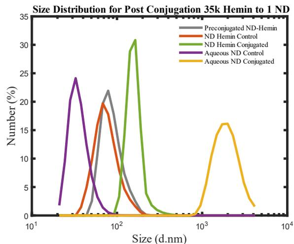
Figure 11. Size distribution of post conjugated nanodiamond-hemin emulsions and aqueous nanodiamond measured via dynamic light scattering.
