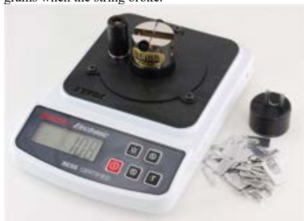
Fig. 3. The Edge-On-Up Industrial Edge Tester
