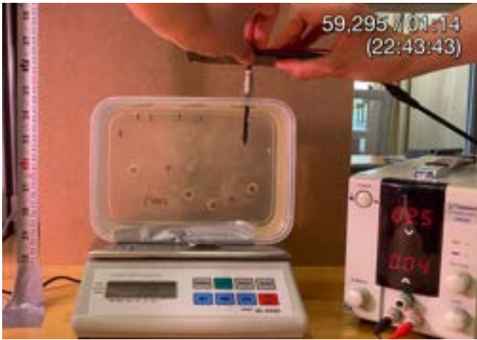
Fig. 4. Image of the testing setup for the tape spring-based needle insertion tests. The 76 kPa gel is positioned vertically above the force transducer, currently measuring a force of 30.4 N. The tape measure on the left, as well as the centimeter lines drawn on the needle itself are used to determine the insertion depth from the videos taken during these experiments. The power supply on the right supplies a voltage of 2.5V to the motor attached to the base of the tape spring needle.
