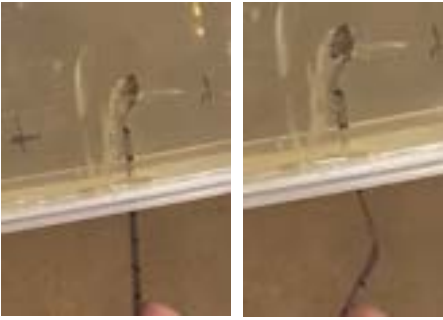
Fig. 6. The image on the left shows a tape spring based steerable needle being inserted straight into a 76 kPa gel. The image on the right shows an instance of the steerable needle buckling in the gel as the result of the needle's insertion or cutting force not being great enough to overcome the gel or tissue stiffness.
