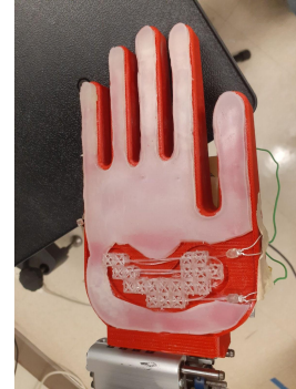
Fig. 4: Photo of Baxter end effector with lossy sensor embedded in palm and silicone.
