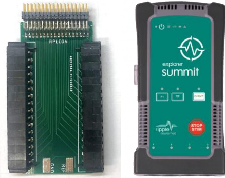
Fig. 6 PCB soldered to connectors (left) and Ripple Grapevine Neural Interface Processor (right). Both components are integral in reducing the amount of wires used drastically. The connectors on the PCB chip snap directly into the blue connectors shown on the MXtrode array in Fig. 4. The Ripple system is connected to the rest of the device via flex cables and will report EMG readings using Bluetooth. Adapted from: Ripple.
