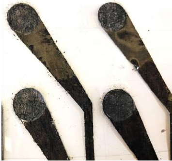
Fig. 5 Close-up image of MXtrode heads after 1 cm biopsy punching. The lower stems of the MXtrode channels are seen to have a glossy sheen, illustrating the presence of the top PDMS encapsulation. The texture at the heads of the electrodes appears rougher as this is where the conductive textile is exposed for skin-interfacing.
