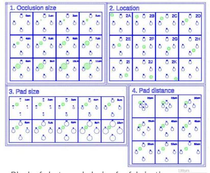
Block of photomask design for fabricating microelectrode arrays defining experiments with occlusions.
