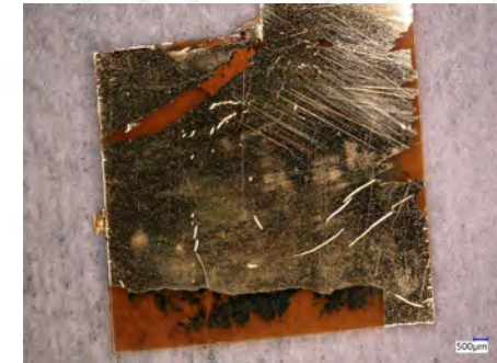
Figure 5: Au electrode in 1e-1 M PBS after voltage of 1.2 V applied
