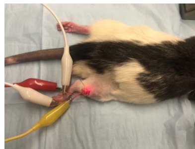
Figure 4. In vivo testing setup. The sensor was coated in clear epoxy and inserted into the hindlimb of an anesthetized rat.
