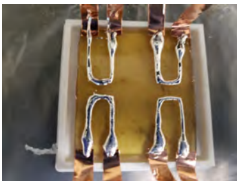
Fig. 13. Simplified strain print before encapsulation
