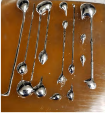
Fig. 8. Printing lines at a height of 0.2 mm above the substrate at increasingly higher pressures from right to left
