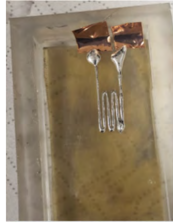
Fig. 10. Strain gauge printed at the optimal print settings prior to encapsulation
