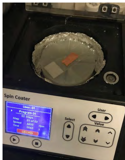
Figure 6. Spin Coater. The sticky orange-brown tape in the center of the rotating platform is where the sample is placed before spin coating.
