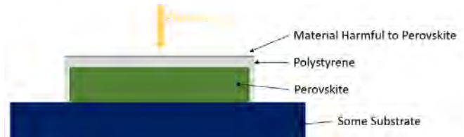
Figure 21. Schematic of why polystyrene may prove useful, if wanting to use material harmful to perovskite in conjunction with perovskite.
