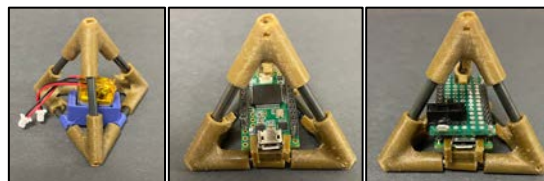
Figure 4: The blue battery mount and brown breakout board connect to the steel springs. These steel springs act as edges between the brown vertices. The middle image shows the Teensy 3.2 breakout board which is 1.4x0.7x0.07in.
