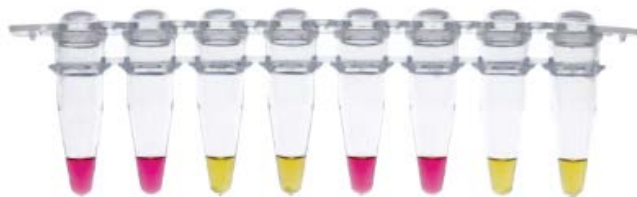
Figure 5 Visual colorimetric detection using pH sensitive dye. With a clear color difference between positive (pink) and negative (yellow) presence of the target template, pH sensitive dyes are a valuable visual detection method. Image from: https://www.neb.com/products/m1800-warmstart-colorimetric-lamp-2x-master-mix-dna-rna#
