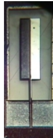
Fig. 1. Single-material Heatuator with selective doping on one arm (G.K. Ananthasuresh)
