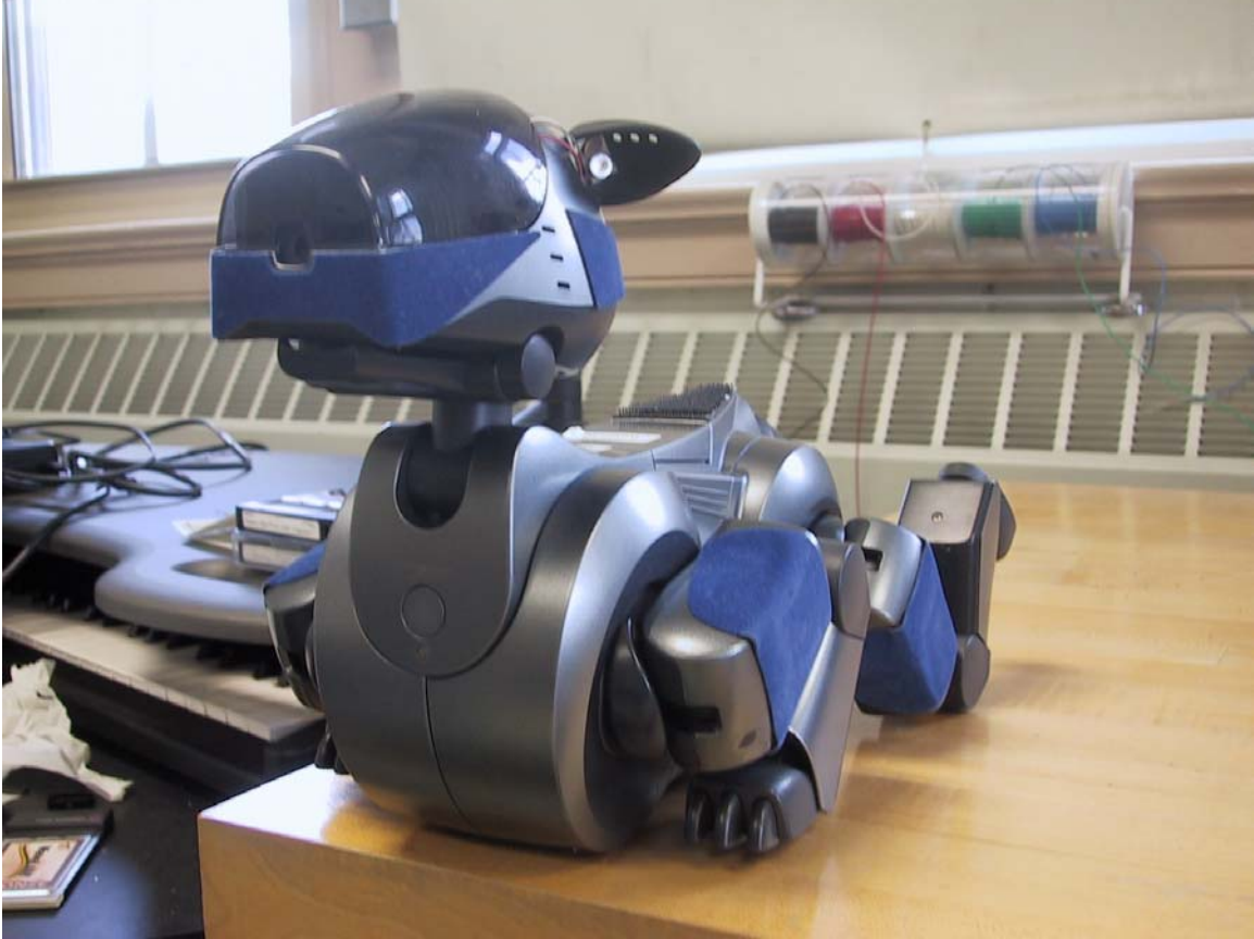
Figure 4: The modified Sony Aibo robot dog. The microphones have been placed inside the “ears,” which now point downward.
