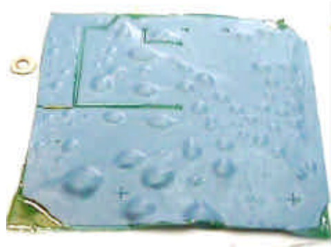
Figure 22: Vias From Figure 18 After Lamination and Full Firing
