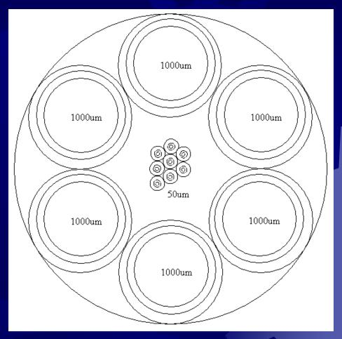
Ideal fiber coupling design shown above would allow maximum transmission of light
