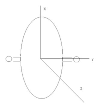
Pitch is defined as rotation around the Y-axis, and yaw is rotation about the Z-axis. Roll, which is rotation about the X-axis, is negated.
