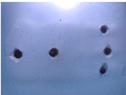
Fig.21 Inlet / outlets on the top laminate of a sintered micro-combustor.
