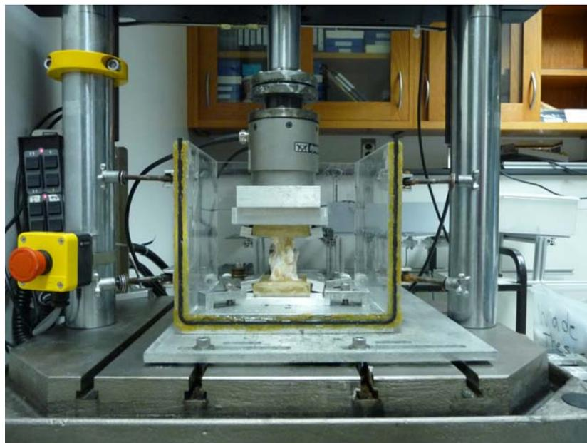
**Figure 8: A picture of the test setup for the preliminary test. This picture does not show the complete PBS bath.**
