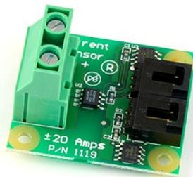
*Figure 4: Phidgets Current Sensor
