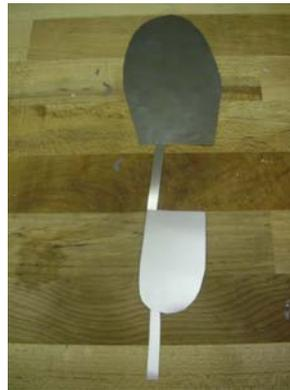
**Figure 5:** Two larger area piezoelectret sensors to be incorporated into the Foot-PAD device.
