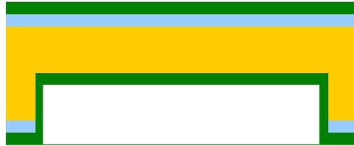
Step 7: Oxide Etching
