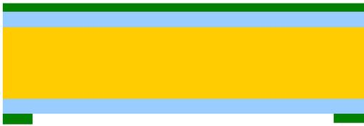
Step 10: Photoresist Layer Spinning
