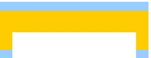
Step 12: UV Exposure of the single axis MM on the top mask
