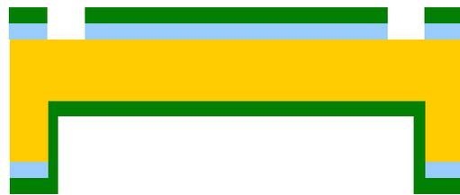
Step 15: Photoresist Stripping
