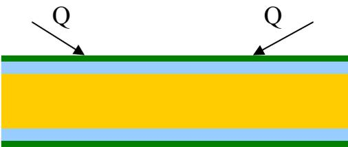
Step 5: UV Exposure of the single axis MM on the bottom mask
