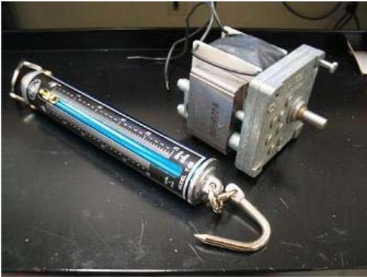
Calibrated Spring and Clock Motor
