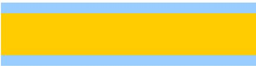
Step 3: Photoresist Layer Spinning
