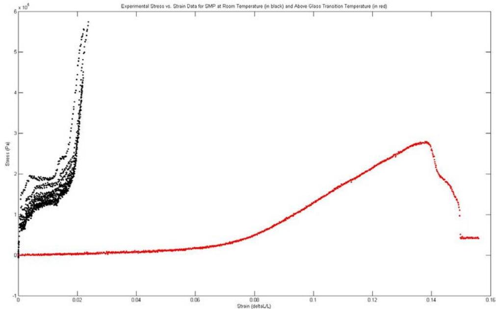
**Figure 15.** Stress Strain Curves for Room Temperature and Heated SMP.
