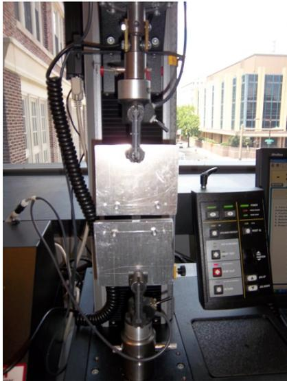
**Figure 4.** SMP sample mounted to aluminum clamps in Instron machine for tensile testing
