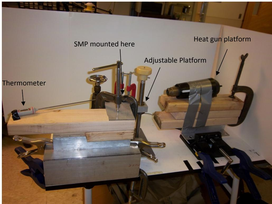
**Figure 5.** Apparatus used for SMP percent recovery testing.
