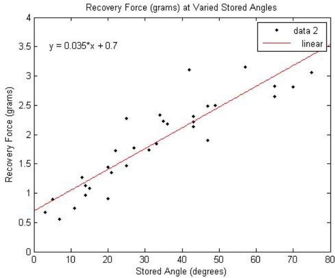
**Figure 18: Recovery Force (grams) at Various Stored Angle Values**
