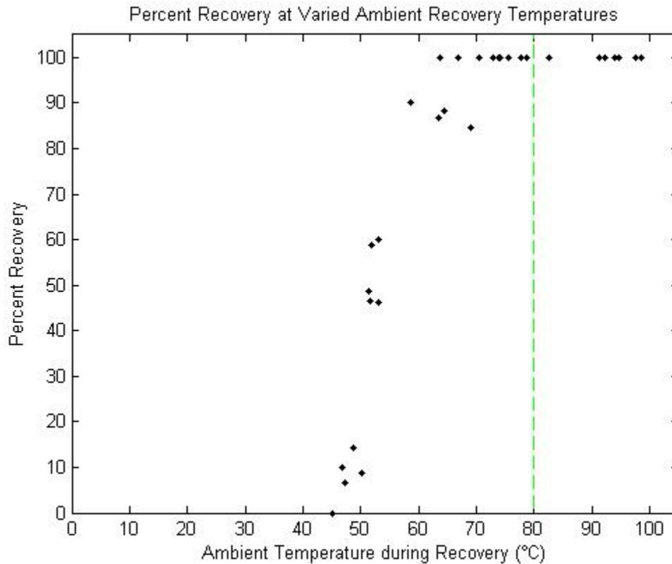
**Figure 16.** Percent Recovery vs. Ambient Recovery Temperature from SMP bending Test.
