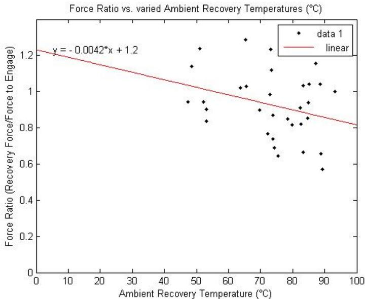
**Figure 20.** Force Ratio (Recovery Force/Force to Engage) vs. Varied Ambient Recovery Temperatures (°C)
