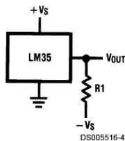
**Figure 2.** Circuitry for LM35 Temperature Sensor.  $V_s=5V$ ,  $R_1=1000\Omega$ . [9]
