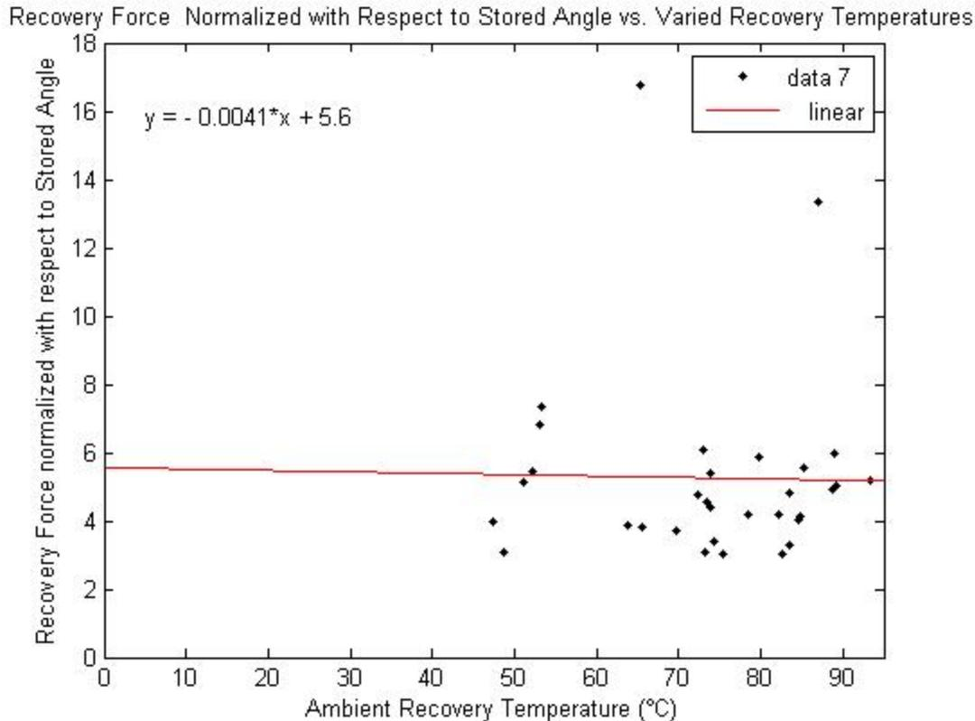
**Figure 21: Recovery Force Multiplied by a factor of Max Angle/Trial Angle vs Various Ambient Recover Temperatures.**
