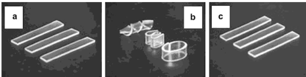
**Figure 1** a) original/permanent SMP shape b) fixed temporary states c) recovered shapes [7]
