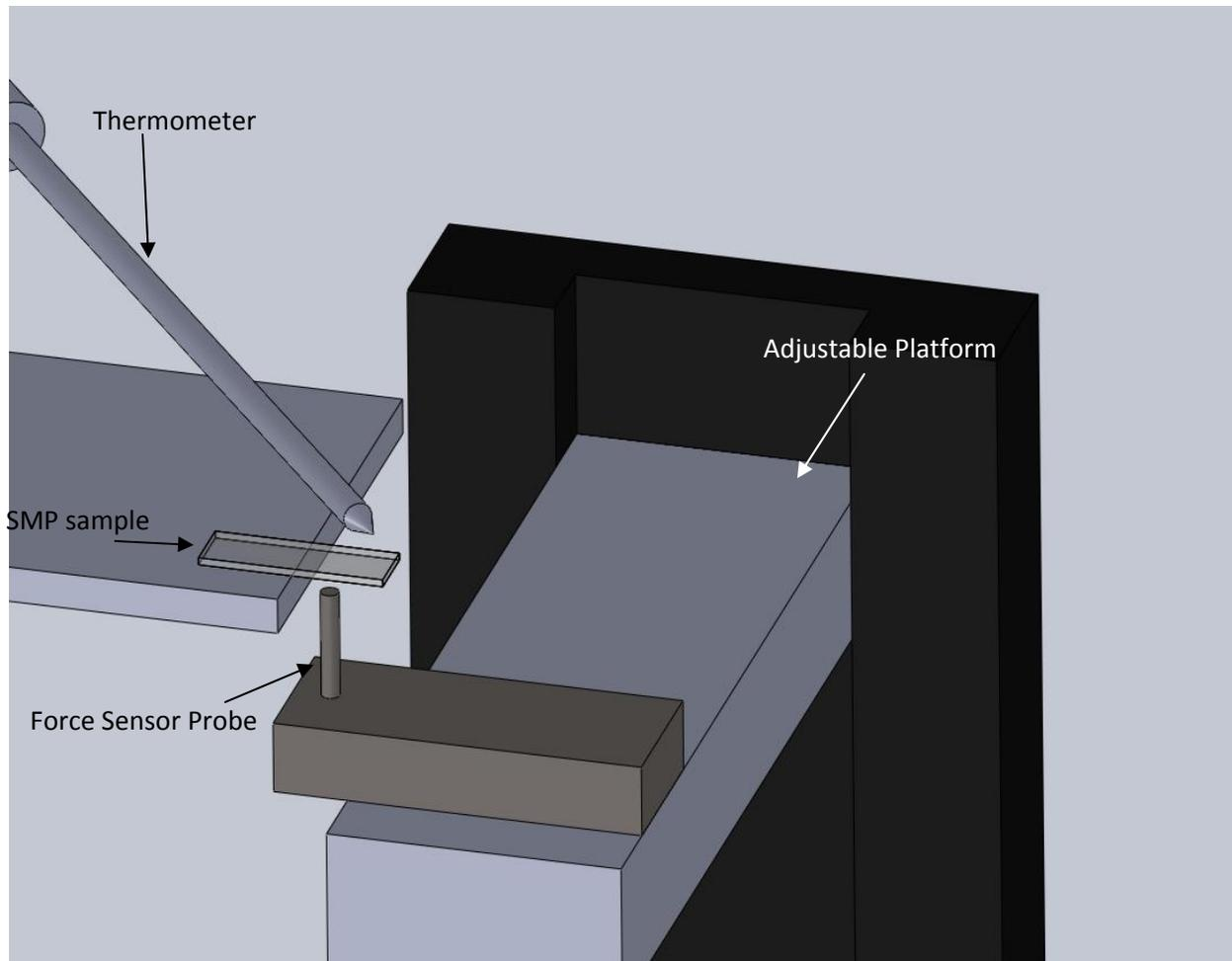
**Figure 6.** Close up of schematic of an SMP sample ready for percent recovery testing.
