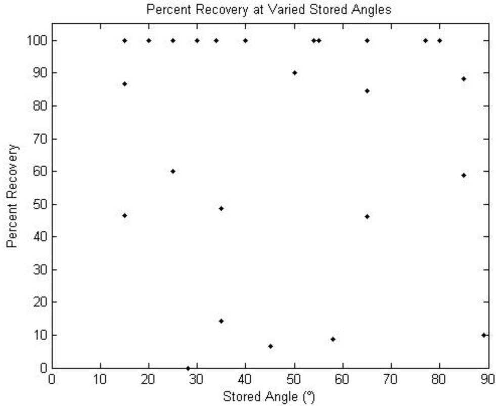
**Figure 17.** Percent Recovery vs. Stored Angle Value for SMP Bending Test.
