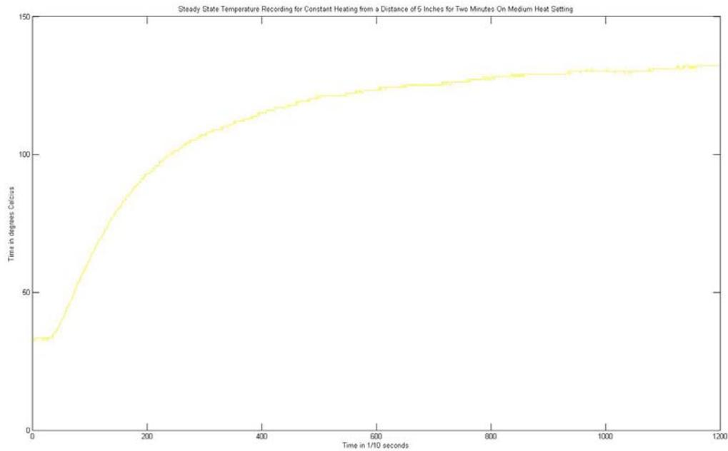
**Figure 9.** Temperature Recording for Medium Heat from a Distance of Five Inches
