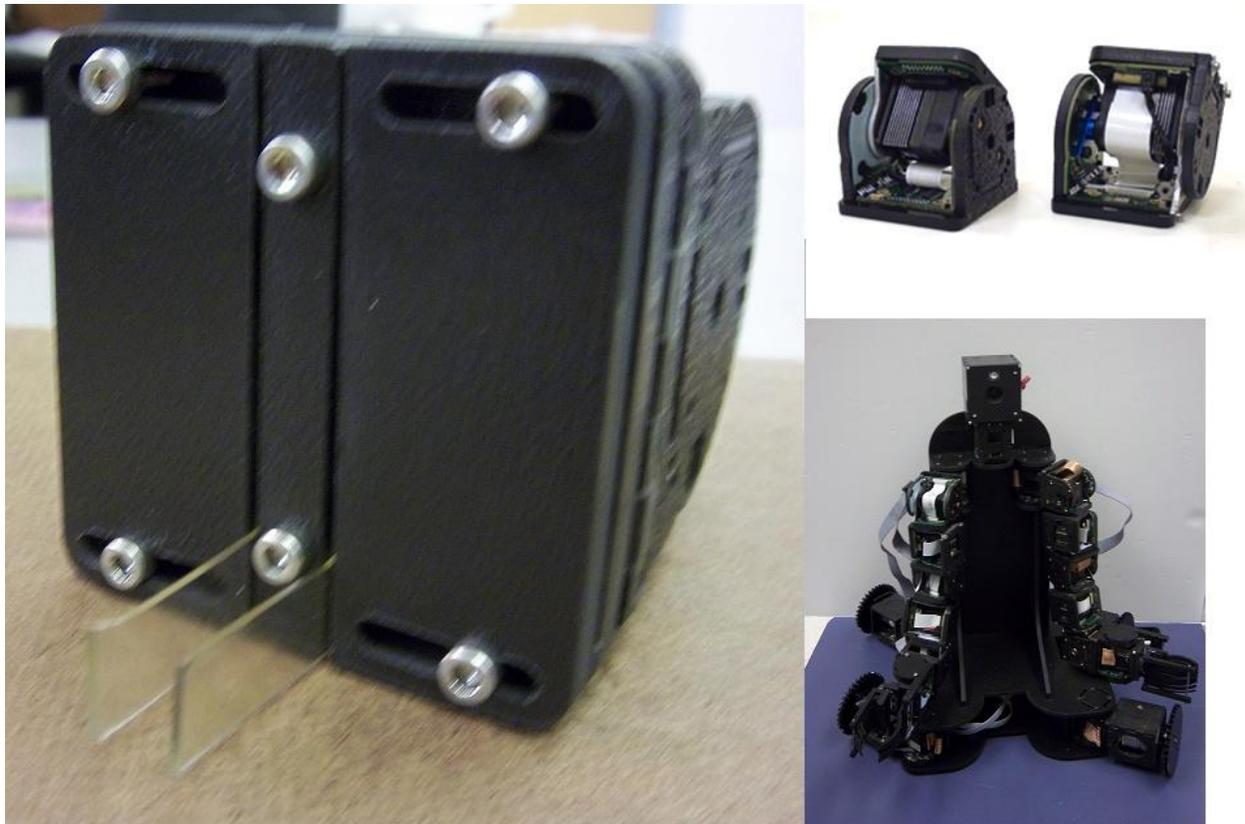
**Figure 8. Left: SMP Gripper, attached to the face of a CKbot module. Top Right: CKbot Modules. Bottom Right: Mini-PR2 robot that was programmed to use the SMP gripper.**
