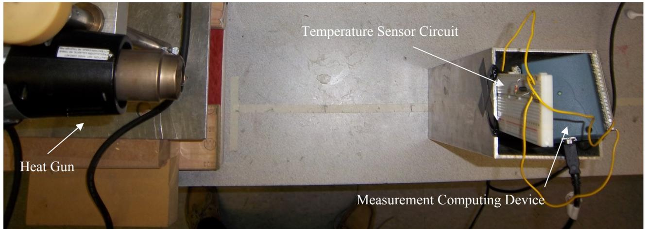
**Figure 3.** Set up for Steady State Temperature Testing
