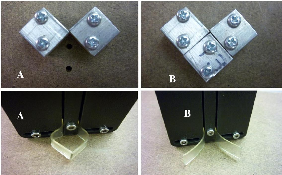
**Figure 22: Two block configurations used to deform the SMP gripper to an open position. Both resulted in successful lifts.**
