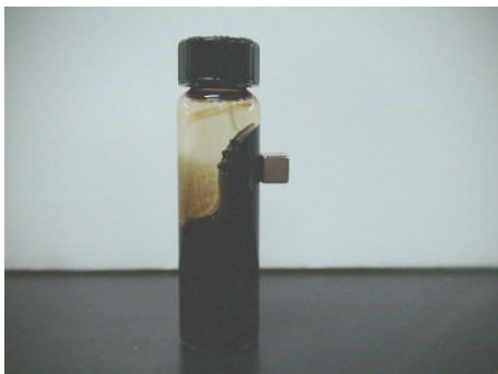
Figure 3. Ferrofluid in vial, with square magnet on side.
