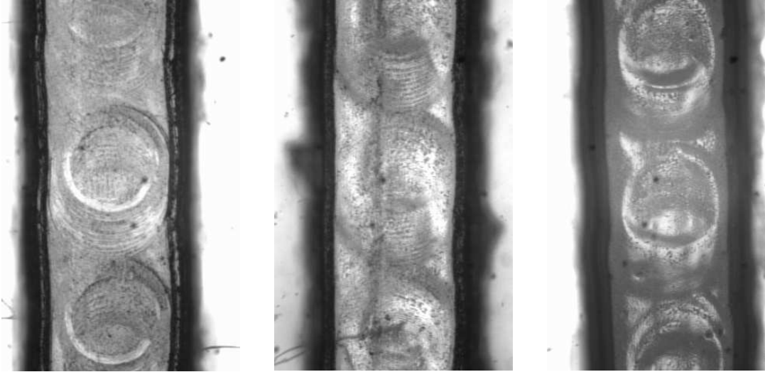
Figure 17. Same channels as above in order: unmodified, acetone applied, PVP treatment (from left to right). 2x magnification
