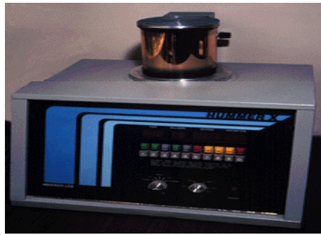
Figure 2: Samples are coated with a very thin layer of either gold or carbon using a Sputter coater. This is done to make a sample conductive so that it could be seen on the SEM.
