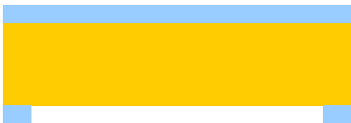
Step 8: Photoresist Stripping
