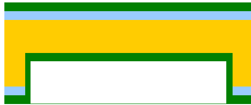
Step 10: Photoresist Layer Spinning
