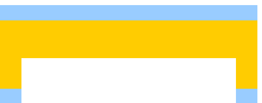
Step 9: Bottom KOH etching
