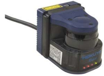
Figure 4: Hokuyo URG-04LX-F01 Laser Scanner (Source: Hokuyo Automatic Co., Ltd.)
