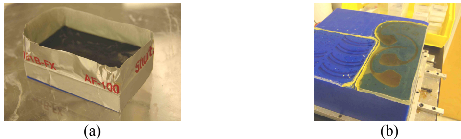
Figure 12: Pour 1 pictures: Example of aluminum tape lining (a), After curing (b). Note the left over yellow modeling clay where a barrier was placed between the two materials.
