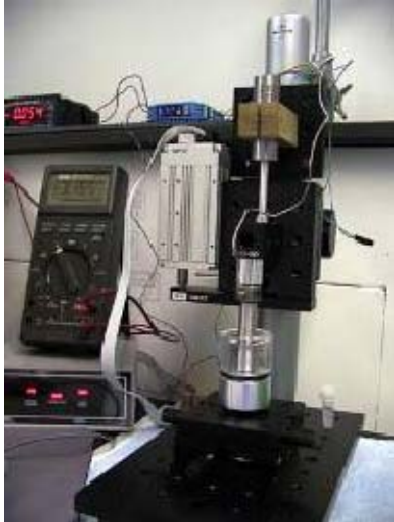
Figure 10. Custom-built confined compression testing device
