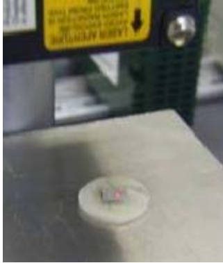
Figure 8. Micro laser sensor used to measure the thickness of samples
