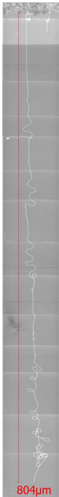
Figure 12: The longest CNT achieved during this project: 804 microns long. Ultra-low gas flow method was employed using a catalyst mixture consisting of Ruthenium Chloride, Iron(III) nitrate, nonahydrate, and alumina nanoparticles of 11nm diameter placed onto silicon chips.
