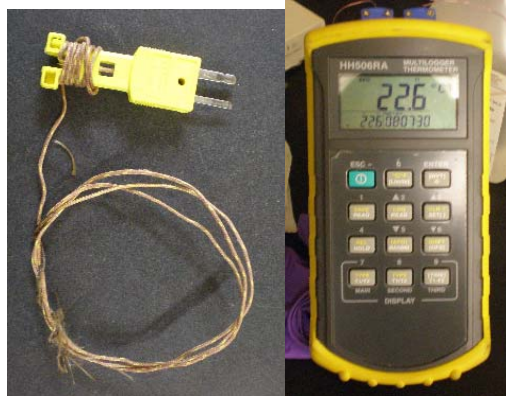
Figure 6: Thermometer (R); thermocouple (L). With the thermocouple attached to a PCR chip, the temperature inside the RT-PCR machine was measured.
