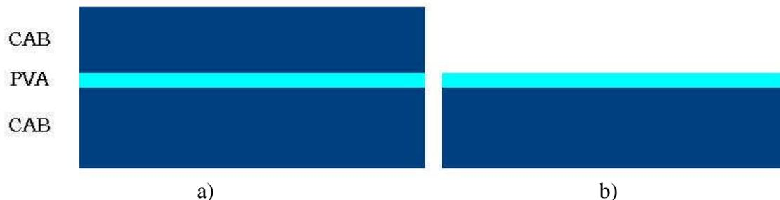
Figure 3: Commercial polarizing filter a) before and b) after the top CAB layer is removed.
