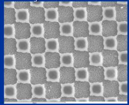
Loss of structure during etching.
