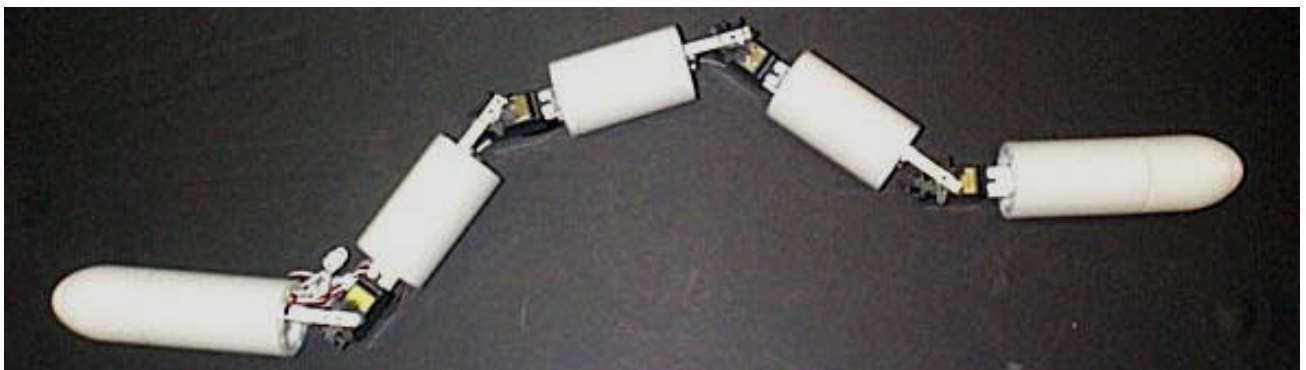
Figure 17. (below) Symmetry of 5-Link Robot, shown fully assembled with nose
