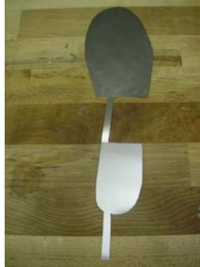
**Figure 5:** Two larger area piezoelectric sensors to be incorporated into the Foot-PAD device.
