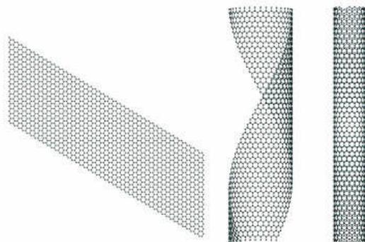
**Figure 2 – Illustration of a graphene sheet being rolled into a carbon nanotube**
