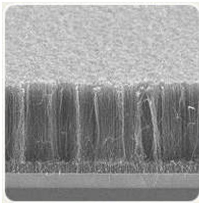
**Figure 6 – An aligned array of carbon nanotubes grown on a silicon substrate**
