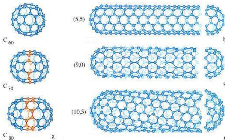
**Figure 3 – Image of armchair, zigzag, and chiral nanotubes (top to bottom on the right) and their corresponding fullerene forms (top to bottom on the left)**
