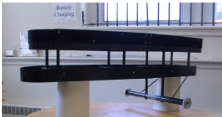
Figure 3: The completed bare carbon fiber gondola.
