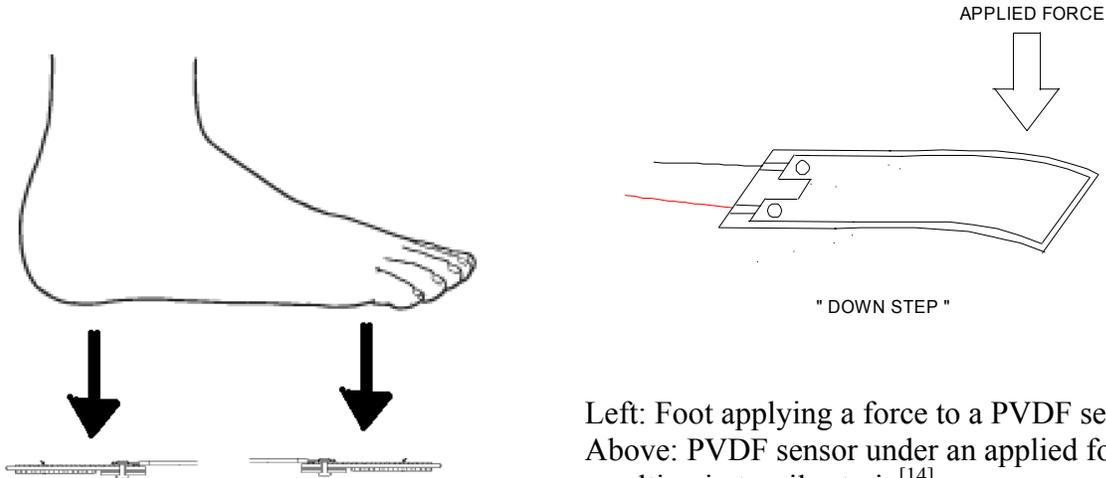
Left: Foot applying a force to a PVDF sensor
