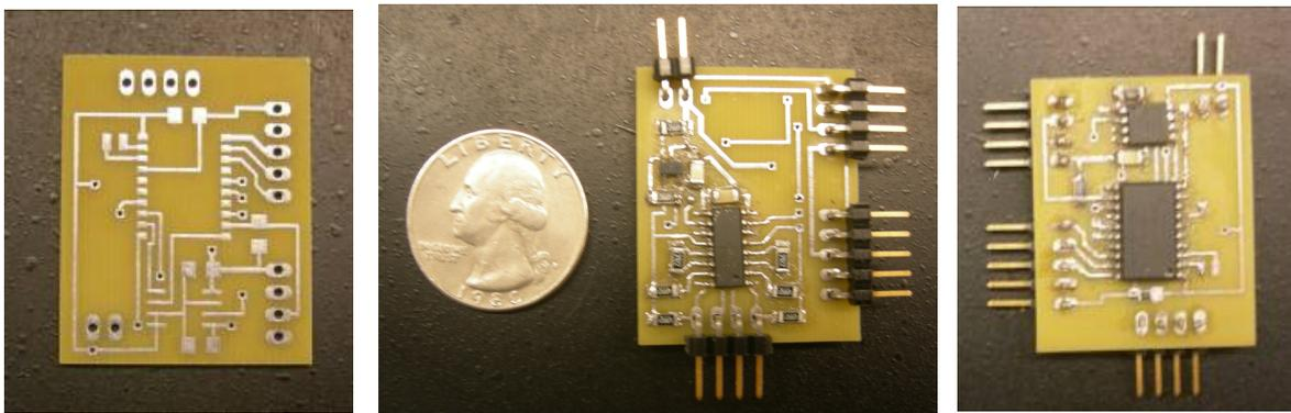
Left: Circuit board of the PD without components (1.125"x 1.406")
