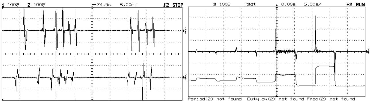
The graph on the left uses the design during a walking exercise. The top function is the sensor at the balls of the feet and the bottom function is the sensor at the heel of the foot. It is clear that the design can obtain measurements during walking.
