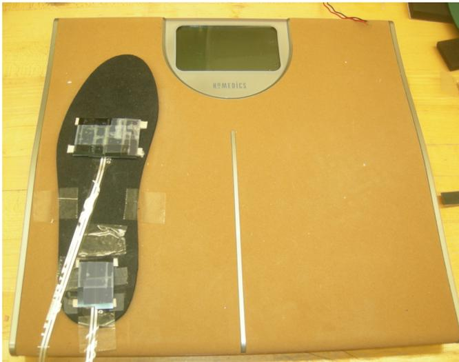
Scale used to measure applied force.
