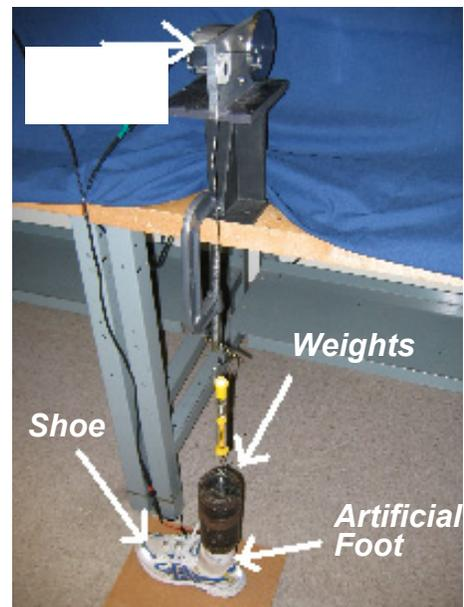
System used to simulate walking.
