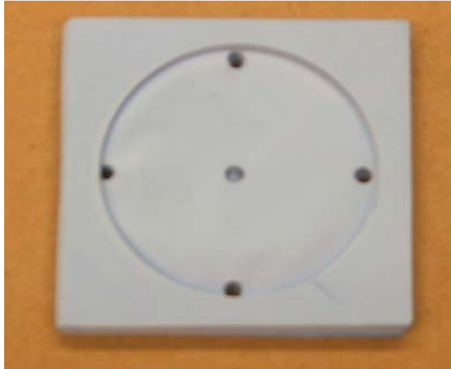
Fig.11 Top view of the micro combustor when the lamination process was done.
