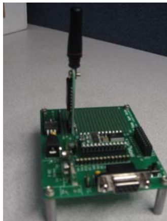
Figure 3: The BASIC Stamp 2 connected to the Parallax 433 MHz RF Receiver
