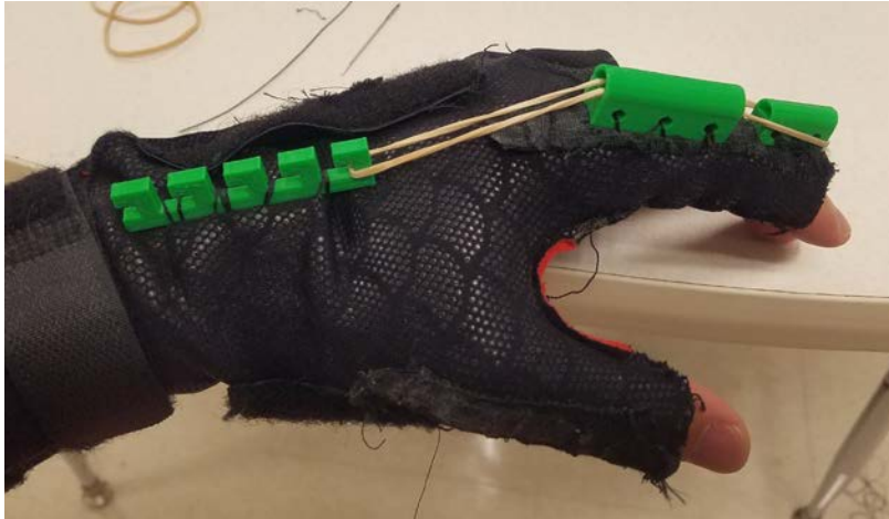
Figure 4: First test of design. The rubber band is directed through the tunnel of the proximal phalanx.
