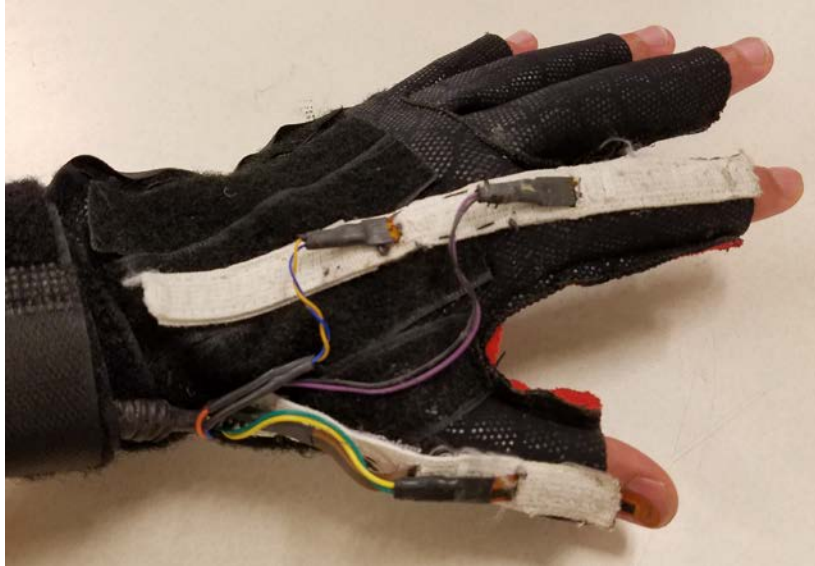
Figure 1: Glove with bend sensors. Four bend sensors measure the angles of the metacarpophalangeal (MCP) and interphalangeal (PIP) joints of the index finger and thumb.
