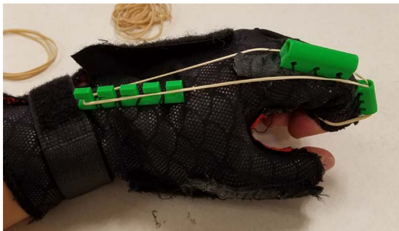
Figure 5: First test with closed hand. The rubber band is instead hooked around the finger to prevent it from flying off. It is also hooked farther away on the back of the hand to test the multiple locations.
