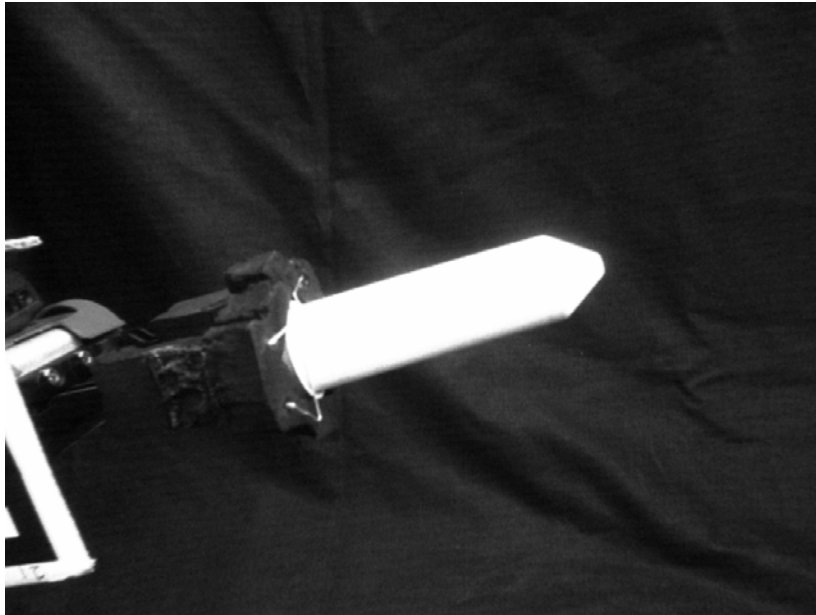
Figure 2: Robot gripper holding experimental test tube
