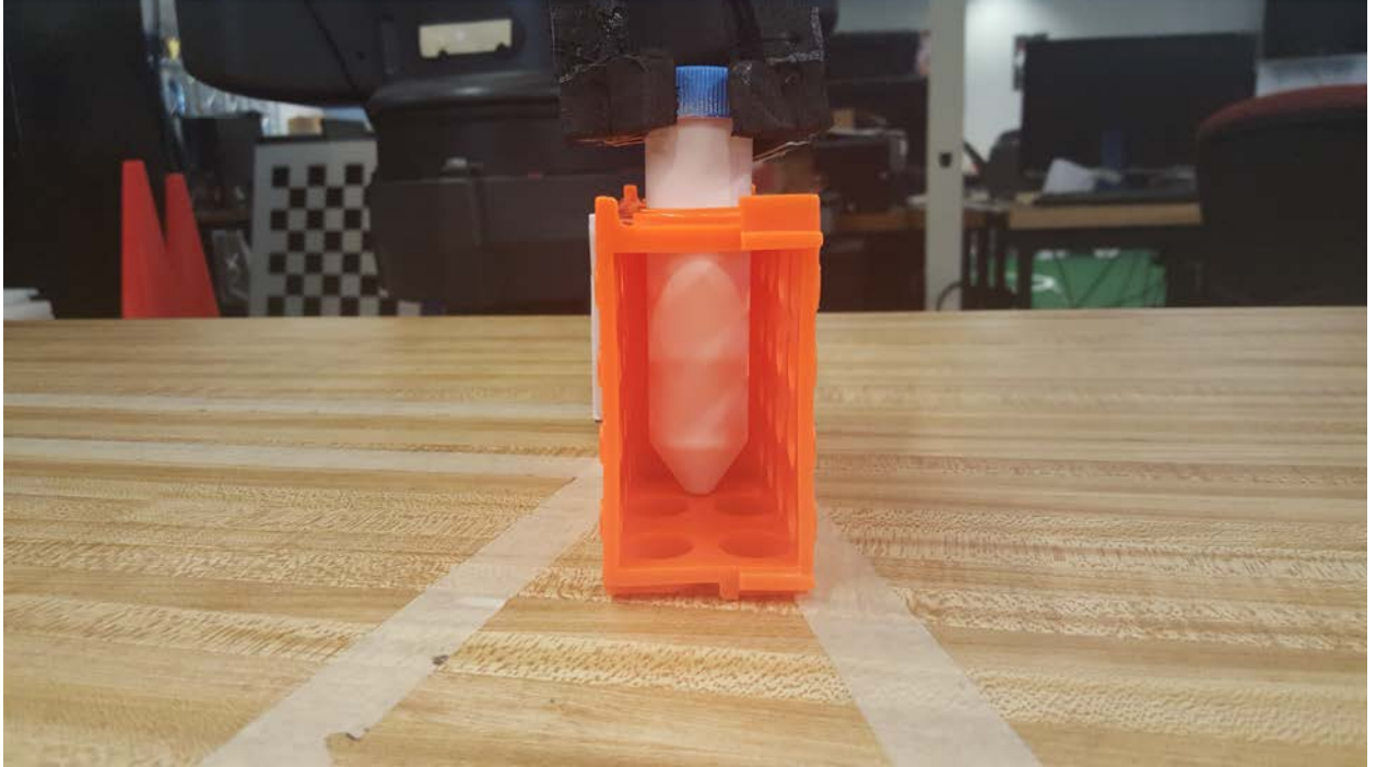
Figure 3. Robot placing a test tube in the array demonstration of peg-in-hole
