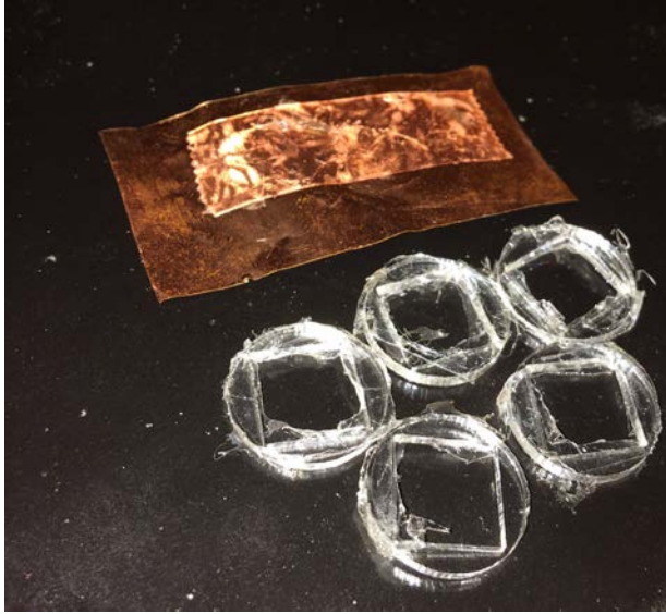
Figure 2. Plastic frames used to collect PVDF films from the PDMS and the copper substrate used to collect the film from the frames.
