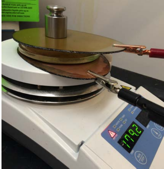
Figure 1. Poling setup used to pole 5% PVDF solution
