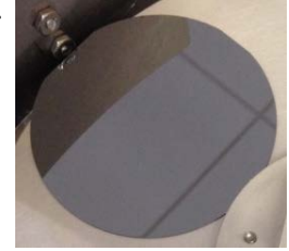
Figure 2: Plain wafer to be deposited with parylene
