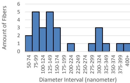
Figure 5a: is a histogram of the frequency of different diameters for the PVDF dissolved in only DMF.
