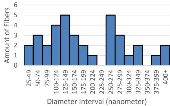
Figure 5b is a histogram of the frequency of different diameters for fibers with F8BT.
