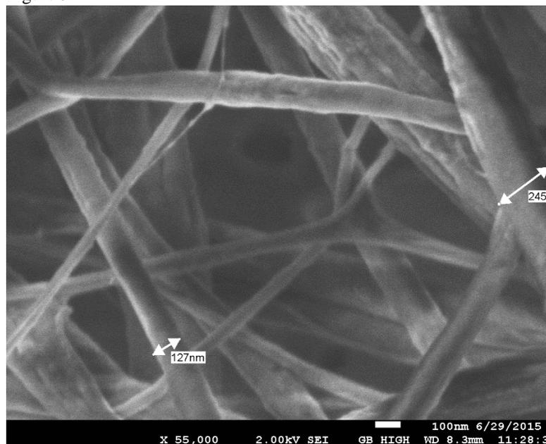
Figure 3 shows the 18 wt. % DMF and acetone solution with F8BT.
