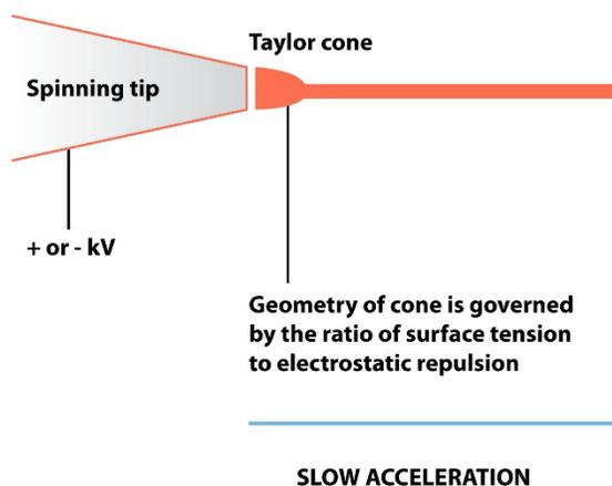
Figure 2b: Illustration of Taylor cone at the tip of a needle
