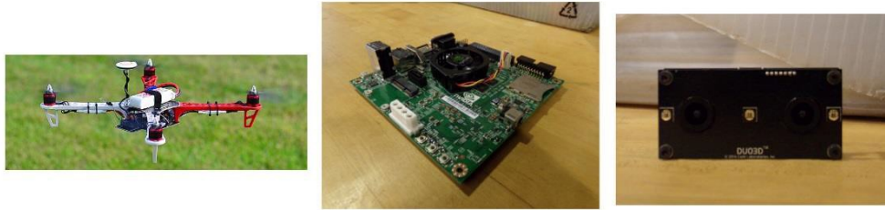
Figure 1 – From left to right: a small quadcopter UAV (DJI F450), the Jetson TK1, and the DUO-MLX. The DUO-MLX has a small 30mm baseline, and a 2.0mm focal length.
