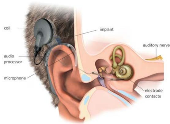
Figure 3 – This picture shows how a cochlear implant looks and how it works.
