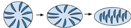
(A) Undeformed, radial (B) Deformed, radial (C) Deformed, no defect present Fig 3d. Cycle of morphology change for droplets
